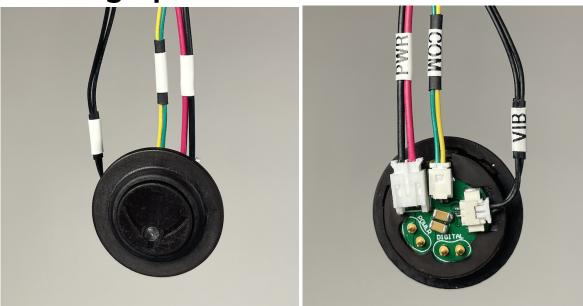
Plug in the **PWR**, **COM**, and **VIB** cables as shown. The **POWER** 2-pin male kidney bean port is used to power the button. The **DIGITAL** 2-pin male kidney bean port is used to connect COAPT. The PSYONIC button can be used with or without an electric wrist.
