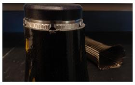
e) Grind down the resin above the lamination cap. Do not grind through the cap. Pry off the cap with side cutters or pliers.
