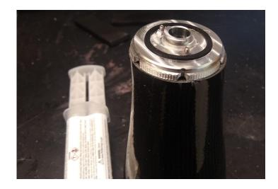
c) Glue the lamination cap onto the socket-side short wrist with hot glue or silicone glue applied to the inside flange of the lamination cap. This seal should prevent resin from seeping under the lamination cap during fabrication. Apply the release agent to the top of the lamination dummy.
