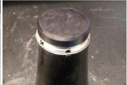
d) Laminate with the desired method. The tie-in point is directly above the knurled section of the socket-side short wrist
