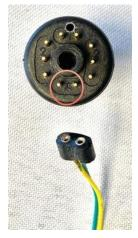
Coapt "OPEN" and "CLOSE" can be plugged into the remaining pins as guided by their manual
