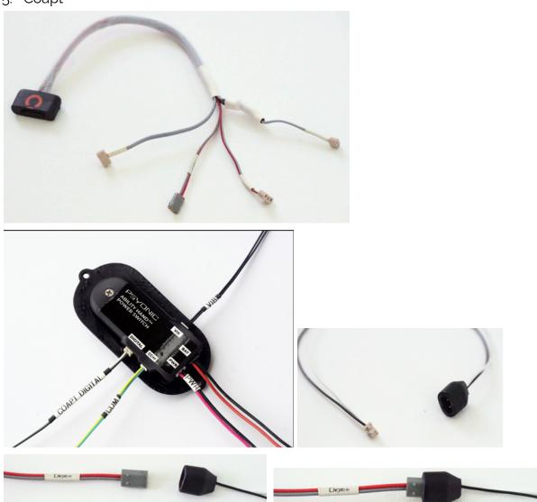
Coapt Digital plugs into black adapter connected to Coapt port on Power Switch
