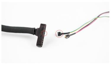
Coapt "OPEN" and "CLOSE" can be plugged into the remaining pins as guided by their manual
