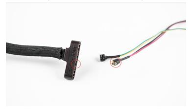
COM (Communication): green/yellow cable from Power Switch to be plugged into the 2-pin half moon end into the second middle port on short wrist connector
