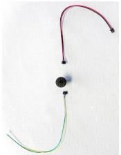
• PWR OUT (Power Out): red/black cable from Power Switch to be plugged into the 3-pin half moon adapter into the "1" port on coaxial plug
