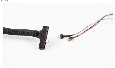
COM (Communication): green/yellow cable from Power Switch to be plugged into the 2-pin half moon end into the second port from the right on short wrist connector
