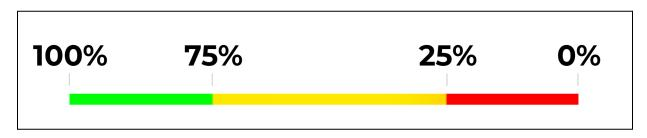
To check the battery status when the hand is in use or not charging, quickly tap the button on the power switch either one time, two times, or three times (Note: the number of times to tap on the button depends on the setup in the app. See App Setup Guide for more information. The color displayed in the LED correlates to the charge level.
